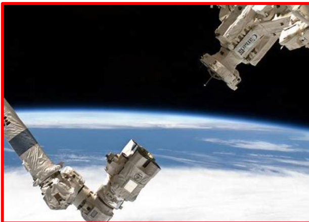
The SSRMS on the left attaching to the Mobile Servicing Systems on the right.
