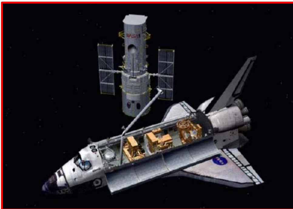
The Space Shuttle Remote Manipulator robot arm and the Hubble Space Telescope.
