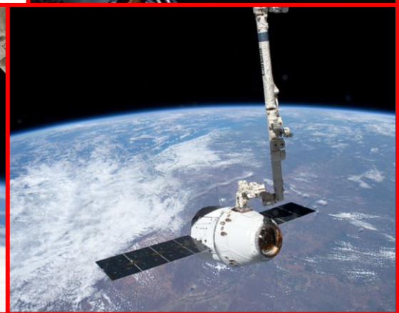
The SSRMS grappling the SpaceX Dragon spacecraft to move the spacecraft to the ISS docking port.
